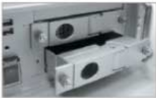
Two Hot-Swappable HDD Drive Bays (HDD adapter boards of IDE or S-ATA are optional)
